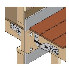
(Part includes bend washer and structural wood screws)
